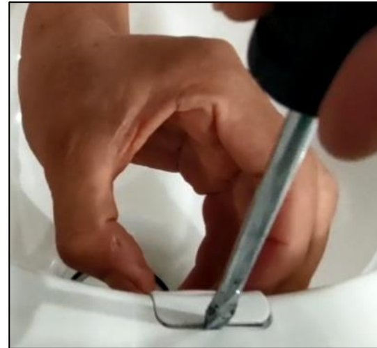
Step 2: Push the cover forward and slide out the cover.
