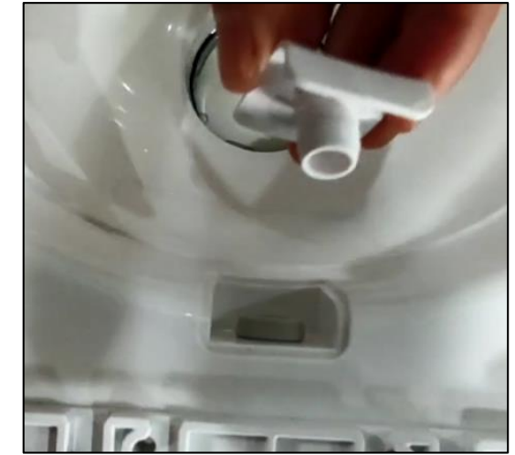
Step 4: Use a flat-blade screwdriver to insert into the gap between the nozzle and the upper housing, and pry out the nozzle.
