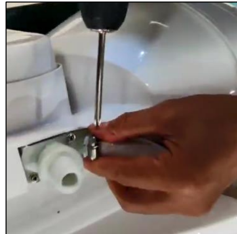
Step 5: Use a cross-head electric hand drill to lock the hose clamp, and the inlet valve kit replacement completed
