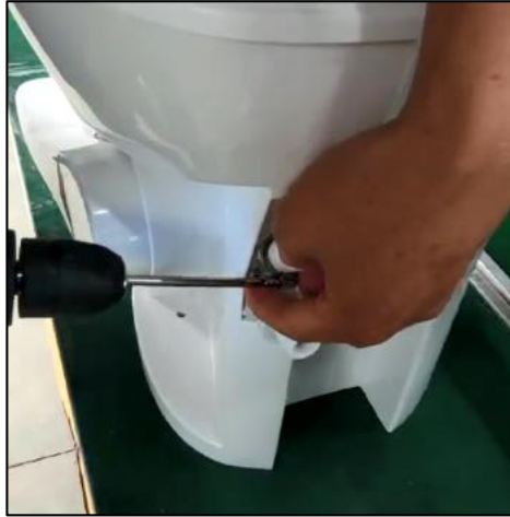
Step 1: Use a cross-head electric hand drill to loosen the outlet hose screw
