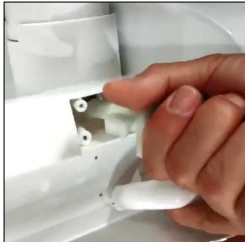
Step 6: Grasp the inlet valve kit, shake it left and right, and then pull it out
